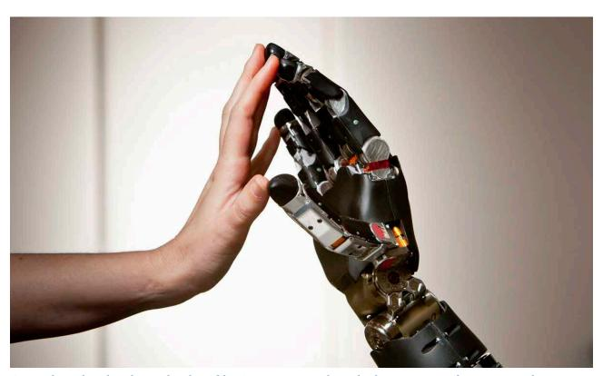
A prosthetic hand and arm developed by APL can not only grab objects as a single movement but can wiggle fingers individually and independently of one another.
